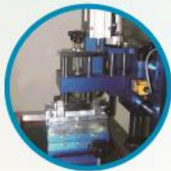
▲ Pneumatic Squeegee Stand / Moving Up and Down
